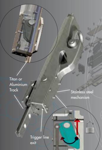
The mainsail locks reduce the mast compression, particularly on maxi-yachts on which working loads are tremendously high. Used on the MOD 70', the Facnor systems reliability has undoubtedly been proved. They can be adapted on existing tracks.
