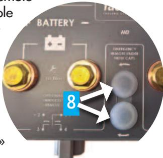
**Note:** the emergency circuit is independent from the control circuit in order to avoid any impact in case of its fusion. In emergency mode : make sure that all safety conditions are respected before handling.
