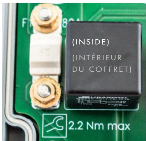
**Caution : excessive tightening torque will destroy irreversibly internal electronic main board.
