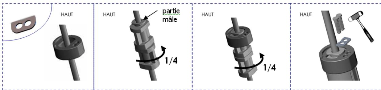
4.2.1- Slip the stainless steel plate and then the top cap around the forestay. Block the plate by slipping it into the notches on the cap, designed for this purpose.
