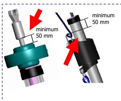
When the sail is hoisted and the halyard is tensioned correctly :
