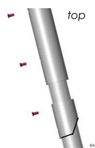
Align holes in the telescopic section with holes in the feeder. Then, screw down the feeder with the screw provided.
