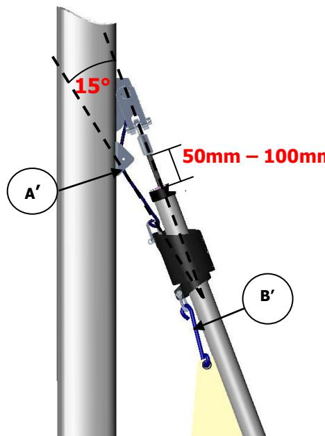
Installation without deflector wheel or when using a sail with shorter luff:
