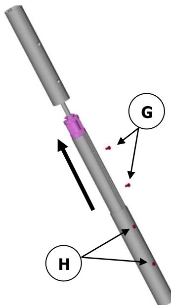
The top section is in place. Assemble a bearing around the forestay. Slip the next section, already assembled (see preparing the sections p.4), with the connector pointing towards the top of the forestay. With the help of the connector, push the bearing all the way up into the top section until the connector holes coincide with those of the top section.
