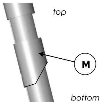
First fit the sail feeder (fig. M) to the telescopic section as indicated.
