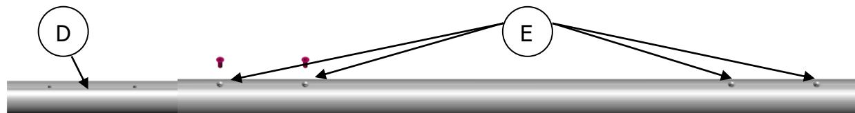
We recommend you prepare the sections before assembly. This involves fixing a connector (fig. D) to all of the twin-groove sections apart from one. The latter will be the top section. All of the external sections, **including the top section\***, have symmetrical holes at each end (fig. E).
