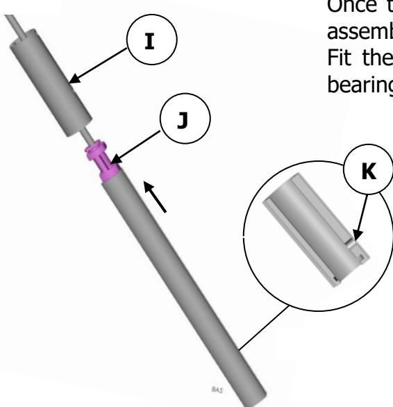
Once the sections have been hoisted as high as possible, assemble a bearing around the forestay.
