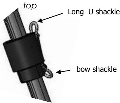
Ensure you fit the halyard swivel the right way up. Fix the two shackles. In order to raise the sections as high as possible, we recommend that you fit the halyard swivel and raise everything by way of a halyard.
