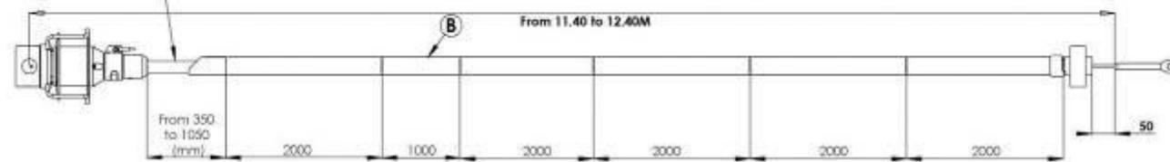
**EXAMPLE No2:** your forestay measures between **11.40 and 12.40 metres**, you do need the 1-metre section (**fig. B**); the latter fits above the last section.
