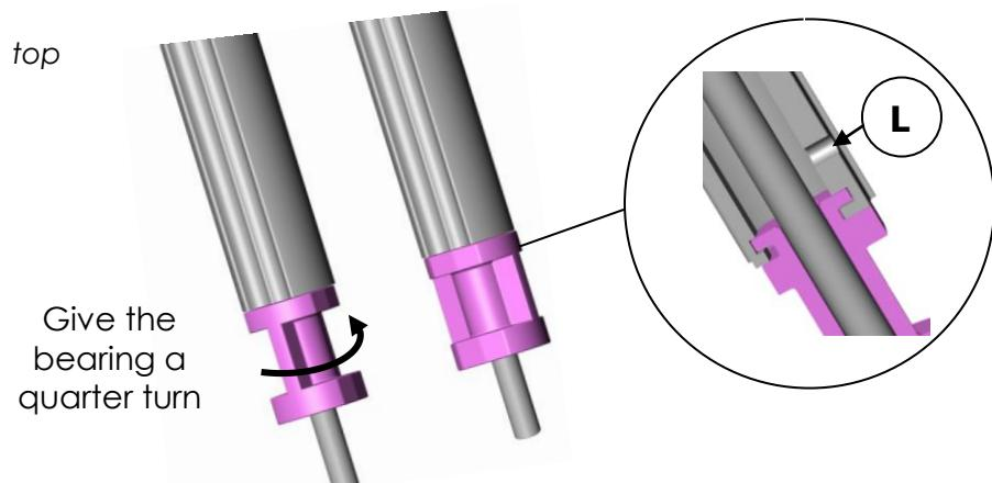
Assemble one bearing beneath the telescopic section, the male side pointing up. Fit the bearing to the telescopic section and give it a quarter turn.
