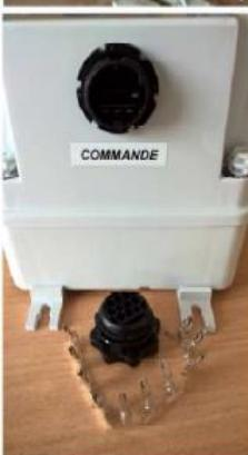
Swage the 5 pins of the remote plug.
