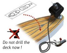
Measure the necessary wire length (L1) to connect the drive unit to the deck socket
