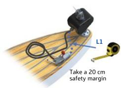
Cut the electric wire (L) at the (L1) distance previously measured (+ 20 cm safety margin)
