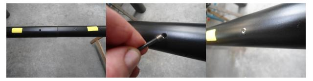
To secure each junction, you'll find a tapered hole in connector and external section. Check before end of glue potlife that these two holes are in front each other. Adjust if necessary. Fit the same araldite glue on supplied screws, and drive the safety screws in place. The screw must be flush to carbon foil external shape. If you drive the safety screw deeper, you may not be able to slide stay and bearings inside the foil.
