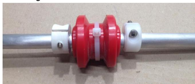
**6- When all the bearings are fitted on the stay, slide it inside the foil.**
