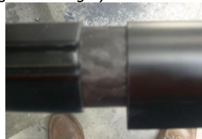
Note: while pushing and twisting the tubes together, the joints need to be cleaned, of any excess adhesive with special attention to the luff groove areas to insure that NO adhesive runs into or between the luff grooves.
