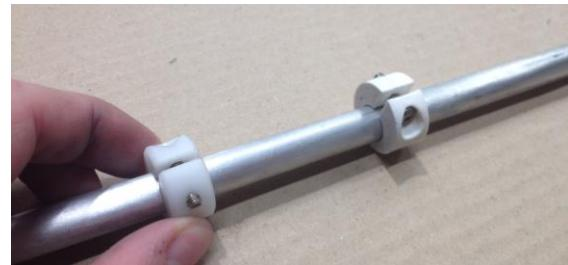
**2-Assemble the two half side stop bushing in the position**
